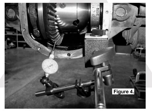
Set a depth indicator on one of the ring gear teeth as in figure 4.
