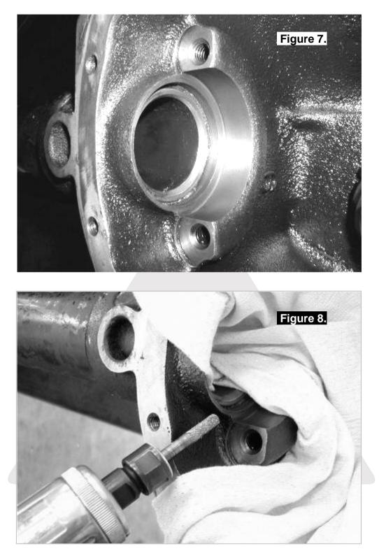
**NOTE :** Cover the differential housing cavity and the axle tube openings with a rag to protect them from metal filings.
