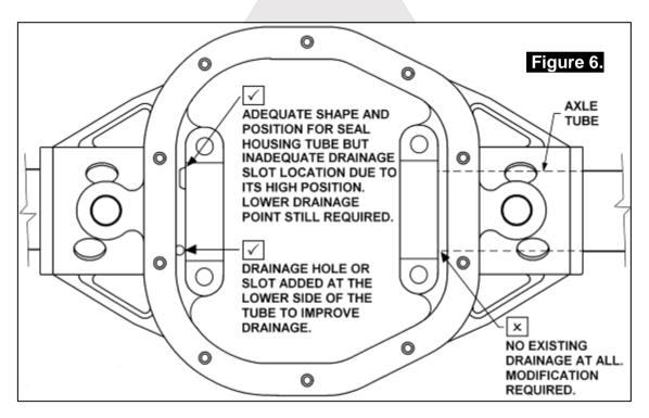
If no drainage exists then two slots should be created in the bearing seat face of both axle tubes; one on the upper side of the tube, and one on the lower side. Figure 7. shows an example of an axle housing with no existing oil drainage.
