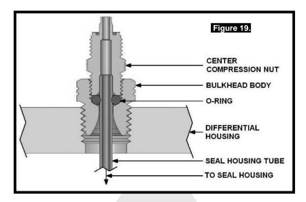
NOTE: Excessive tightening of the center compression nut is not necessary to form a good seal around the tube and may damage the O-ring, the seal housing tube, or the threads of the compression nut.
