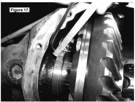
NOTE: The seal housing tube should lay as low in the seal housing groove as possible.
