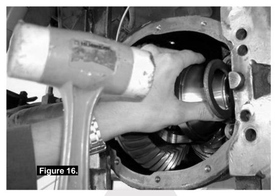
NOTE: If the master shim is too tight to fully install then the spreader tension may need to be increased. Do not spread the housing more than 0.50mm [0.020"].
