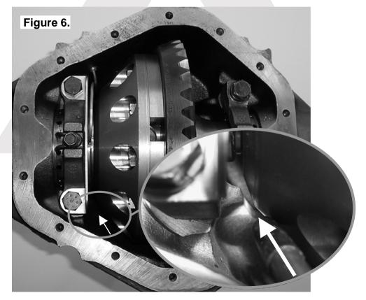
Once the required clearance has been achieved thoroughly clean the axle housing of any grinding dust or other foreign particles.
