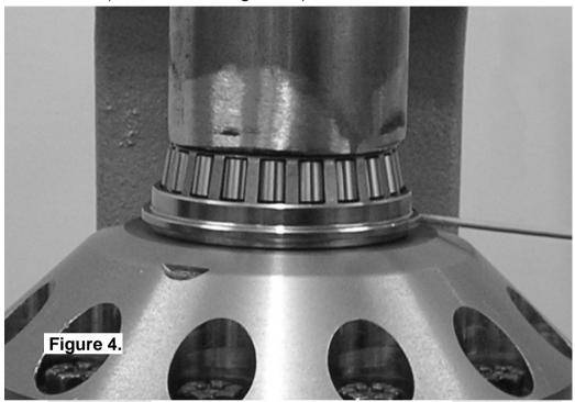
Invert the *Air Locker* and press the other tapered roller bearing cone onto the opposite bearing journal of the differential carrier until the bearing seats firmly against the bearing journal shoulder.
