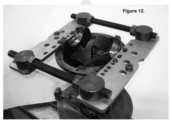
☐ Carefully spread the housing (Fig 12.) just enough to install the differential carrier (Refer to your vehicle's service manual).
