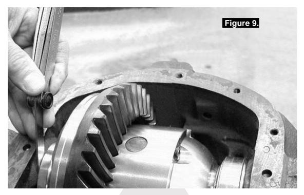
Add the specified preload amount to the end float measurement determined with the feeler gauge to determine a shim amount for 'E' (Refer to Figure 7.).
