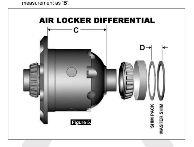
☐ Measure the distance from the *Air Locker* bearing shoulder to the ring gear mounting face (shown as '**C**' in Figure 5.) and record this measurement as '**C**'.
