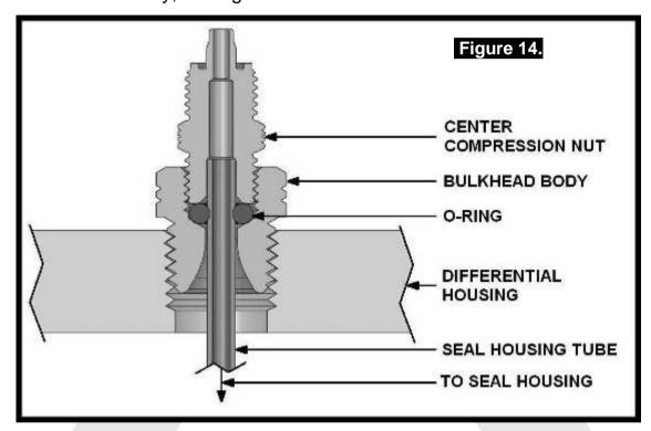
NOTE: Excessive tightening of the center compression nut is not necessary to form a good seal around the tube and may damage the O-ring or the threads of the compression nut.
