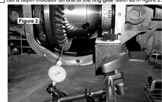
Set a depth indicator on one of the ring gear teeth as in figure 2.
