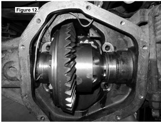
NOTE: It is also a good idea to keep the tube away from the bearing caps or any other part of the differential casting as any contact due to vibration or shock may wear the tube and eventually cause a leak.
