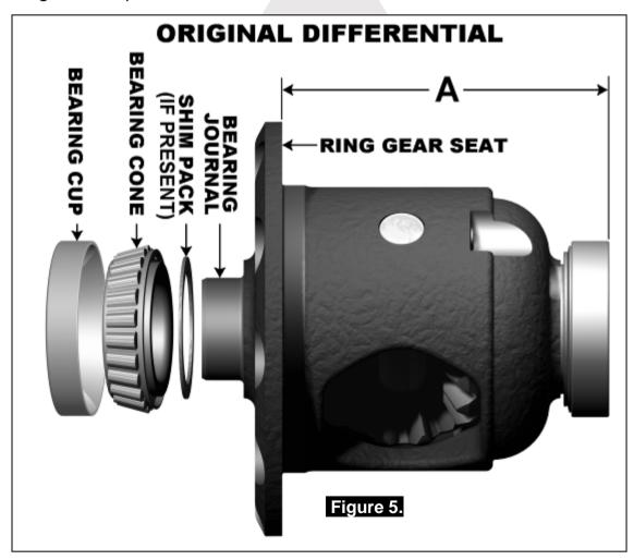
Assemble the original bearing cup onto the cone of the right-hand side of the original differential carrier.
