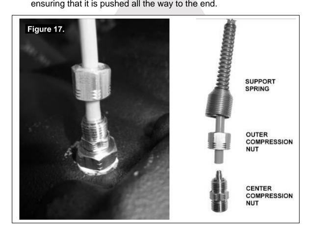
HINT: If the tube is too difficult to push on, place the end of the air line into a cup of boiled water to soften the tubing.
