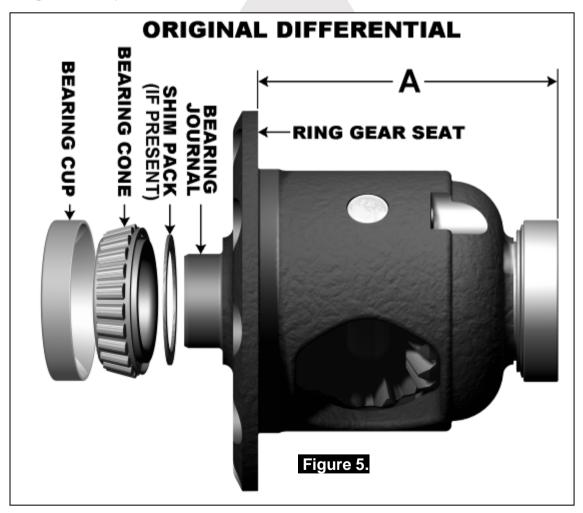
Assemble the original bearing cup onto the cone of the right-hand side of the original differential carrier.
