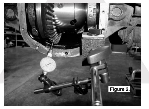
Set a depth indicator on one of the ring gear teeth as in figure 2.
