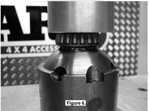
Invert the Air Locker and press the other tapered roller bearing cone onto the opposite bearing journal of the differential carrier until the bearing seats firmly against the bearing journal shoulder.
