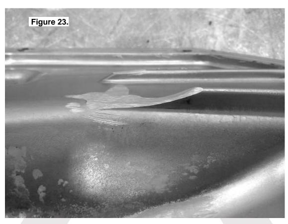
Replace the differential cover using gasket sealant or a new standard differential cover gasket for your make of vehicle.
