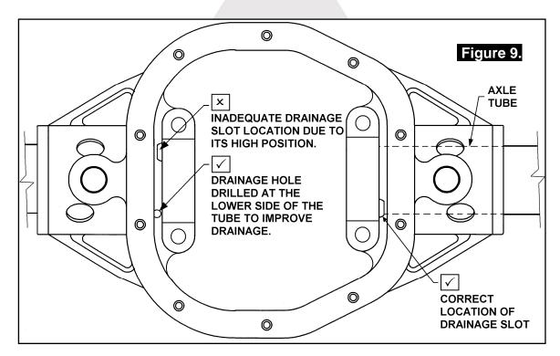
If drainage exists but is inadequate then a slot or hole should be cut into the housing on the lower side of the tube(s) to allow oil out of the axle tube area.
