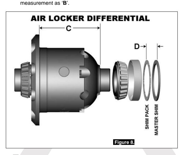
☐ Measure the distance from the *Air Locker* bearing shoulder to the ring gear mounting face (shown as 'C' in Fig.8.) and record this measurement as 'C'.
