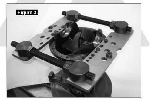
Release all spreader tension immediately after removing the differential carrier.
