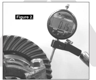
Set a depth indicator on one of the ring gear teeth as in Figure 2.
