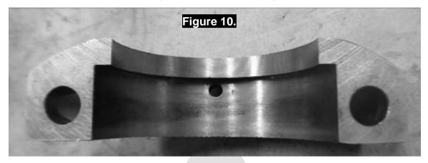
**NOTE :** Take time and double check when drilling, as bearing caps are custom fitted to the diff housing and cannot be replaced.
