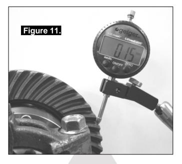
Refer to your vehicle service manual for the specified maximum and minimum amounts of backlash. If the backlash is not within the specifications then the differential will have to be removed and reshimmed.
