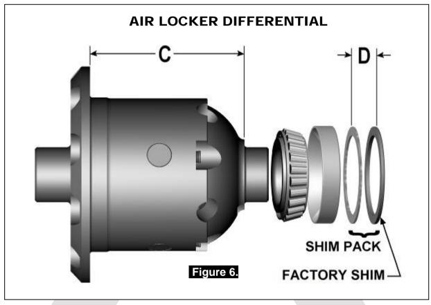
Measure the distance from the Air Locker bearing shoulder to the ring gear mounting face (shown as 'C' in Figure 6.) and record this measurement as 'C'.
